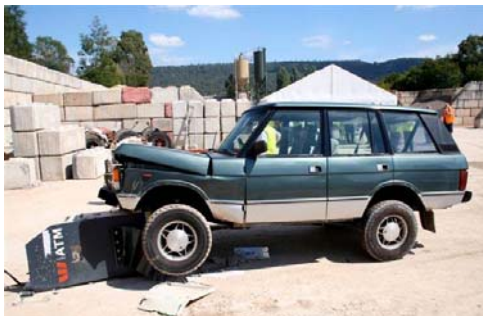
An ATM safe under repeated ram attack test. The safe remained attached to the Raminator.
